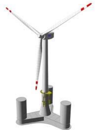
OO-Star, steel or concrete
