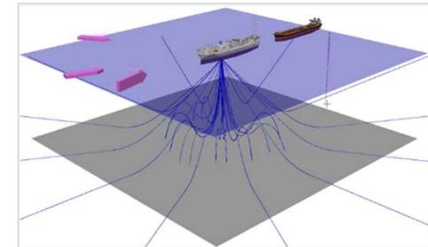
Calculation of operational limits for hawser-less offloading operation
