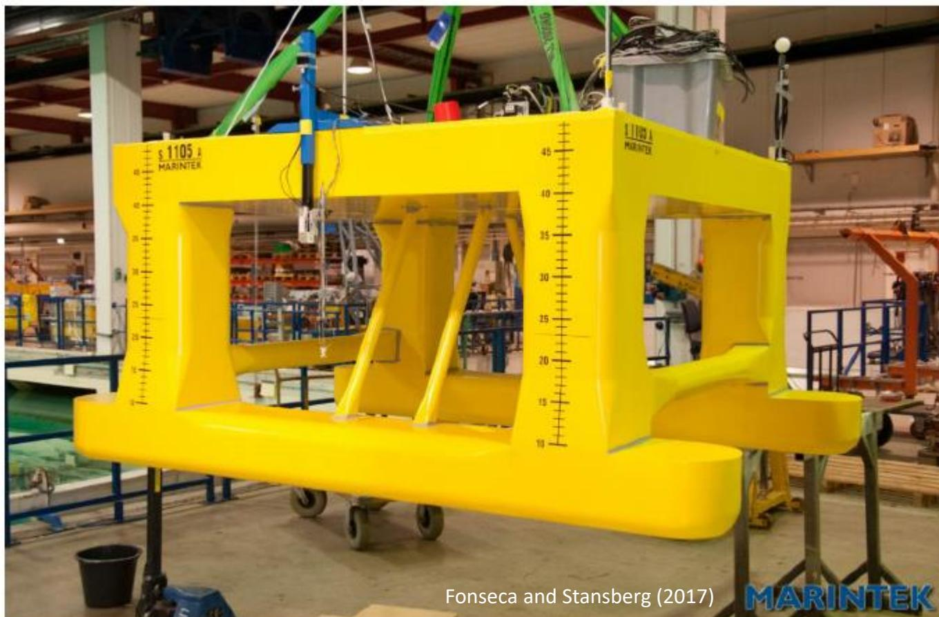
Figure 1: EXWAVE semi-submersible 1:50 scaled model.
